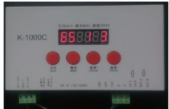
6. Please press and hold the "CHIP" key first, then press the "MODE" key at the same time to exit the addressing mode and enter the controller mode, as follow picture shows:
