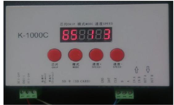
4. Press "MODE" and start to address the strip, "A A A" will be shown on the controller, as follow picture shows:
