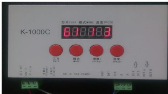
3. Press "CHIP" key to adjust the first and second displayed value to "65", the final value should be kept at "3" ( If it is not number "3" but other value, it can be adjusted by the two keys of SPEED+/-SPEED- ). As follow picture shows:
