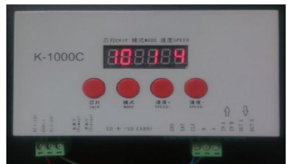
7. The first and second displayed value must be "10", if it's not, the strip couldn't be controlled normally. The two value can be changed by adjusting "CHIP" key.
